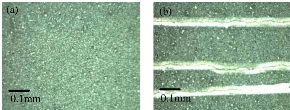
Fig.5 Photograph of typical surface of Cu(In,Ga)S<sub>2</sub> film in condition shown by (a) and ×(b) in table 1.
