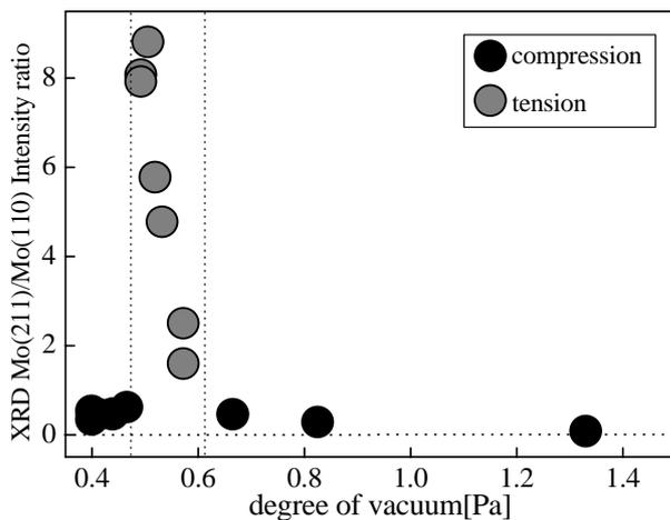
Fig.3 (211) XRD intensity of Mo film deposited on polyimide substrate normalized to the (110) intensity as a function of degree of vacuum during deposition
