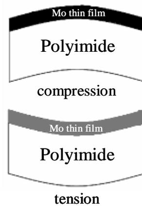
Fig.4 Schematic drawing of the Mo films on polyimide substrate of compression and tension condition.
