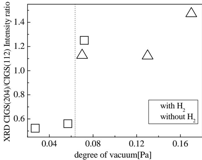
Fig.2 (204) XRD intensity of Cu(In,Ga)S<sub>2</sub> film normalized to the (112) intensity as a function of degree of vacuum during deposition
