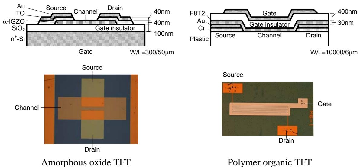
Fig. 1 Device structures of the amorphous oxide TFT and polymer organic TFT.
