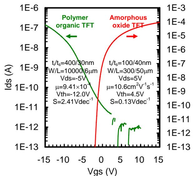
Fig. 2 Transistor characteristics of the amorphous oxide TFT and polymer organic TFT.
